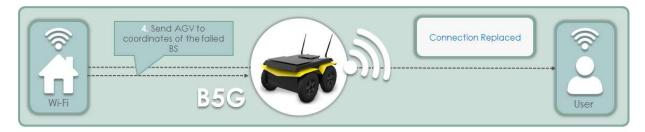
Figure 23: High-level view of Jackal being used as a MAP
