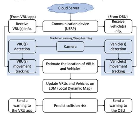
Figure 34: The overall software structure of the proposed RSU
