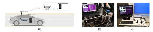
Figure 36: SDR-based V2X communication device on TUC vehicle platform: (a) installation setup (b) UE (c) CN+eNB
