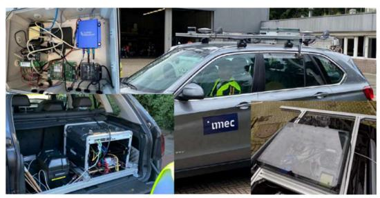
Figure 32: IMEC's experiment car with On-board Unit
