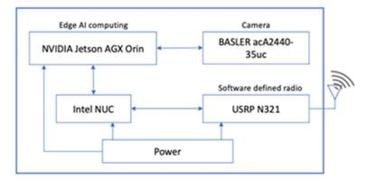
Figure 33: RSU prototype hardware configuration
