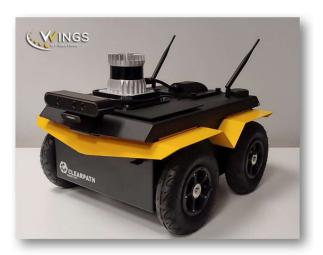
Figure 21: Clearpath Robotics Jackal Unmanned Ground Vehicle
