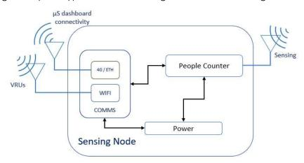
Figure 38: Sensing node prototype
