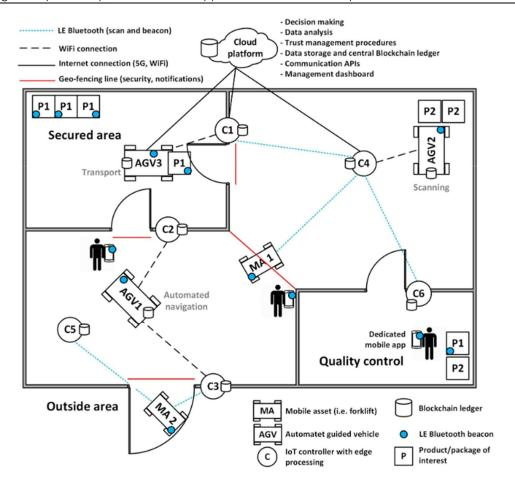
Figure 7: Smart warehousing use case setup plan
